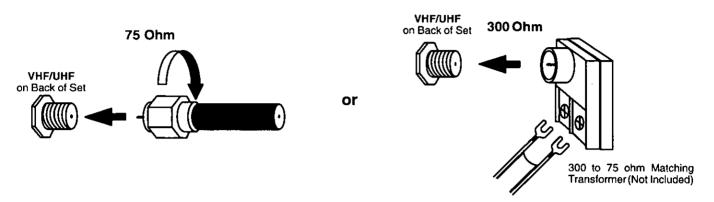
**Cable Connection** – For reception of cable channels, connect the cable supplied by your local cable company. **Antenna Mode must be set to CABLE.** (Refer to Antenna Mode section.)
